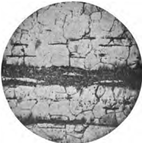
FIG. 13. — Wrought Iron. Longitudinal Section. Magnified 100 Diameters. (Boynton.)
